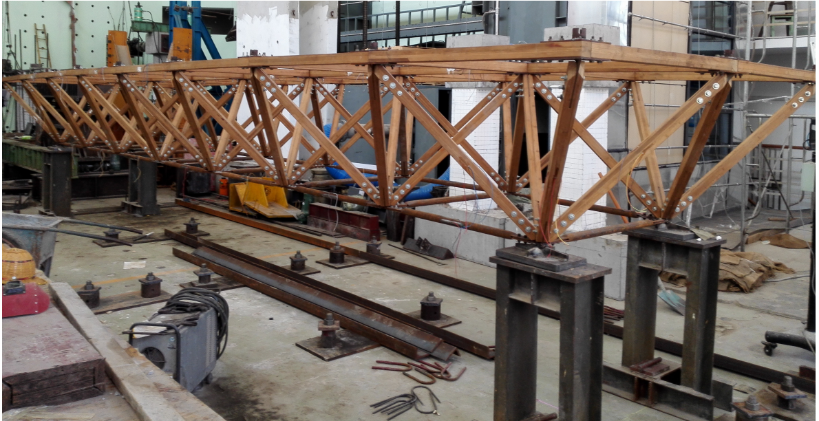
Figure 1: Tested composite glulam-steel truss structure.
