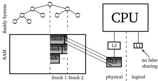
Figure 4: `posix_mem_align` behaviour
