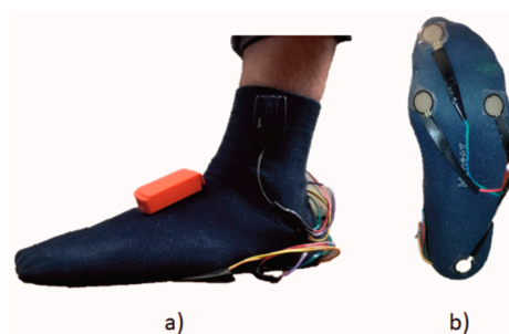
Figure 1. Sensors positioning on subject. (a) Position of IMU on participant's foot; (b) position of footswitches under participant's foot.
