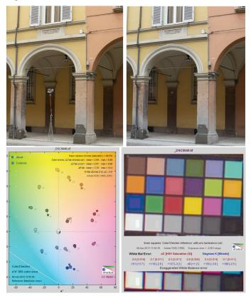
Fig. 8 Upper image: Gretag ColorChecker picture setup with and without a target; lower image, left: mean camera chroma relative to the mean ideal chroma in the CIE colour metric ( $\Delta E^*ab$ ) for the colour balanced image; lower image, right: colour analysis for the same colour balanced image.
