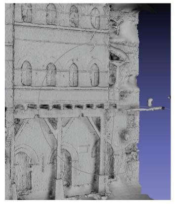
Fig. 6 The mesh of a portion of porticoes from our process.
