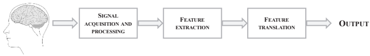
Figure 1 - Overview of a BCI system. EEG signals, acquired from the scalp, are processed and analysed to extract specific signal features. These features are translated into commands that operate a device or feedbacks provided to the subject.
