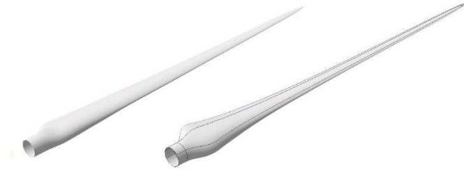
Figure 3. Blade surface. Left: Baseline blade; right: Optimized airfoils blade.
