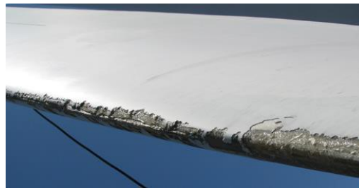
Figure 1. Leading edge erosion [3]
