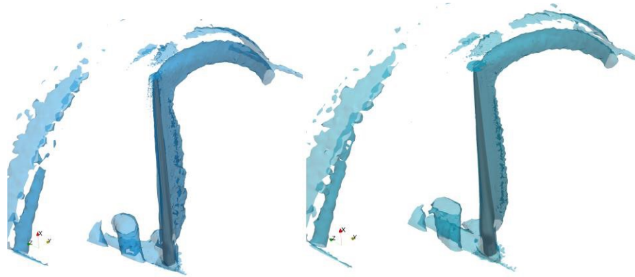
Figure 5. Vorticity iso-surface. Left: Baseline blade; right: Optimized airfoils blade.
