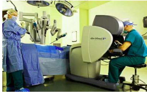
Figure 1.4. Surgeon operating with the da Vinci robotic system observes the clinical scene with the 3D vision system of the master console.
