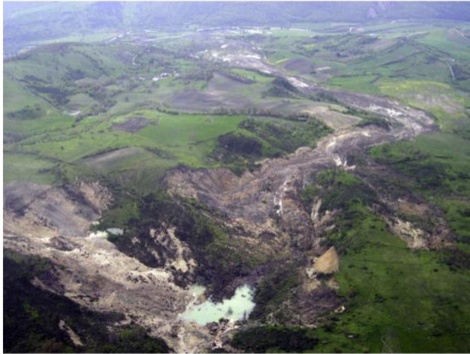
Figure 22 - Main scarp of Montaguto earthflow (view from the top) (source: Guerriero et al. , 2014)
