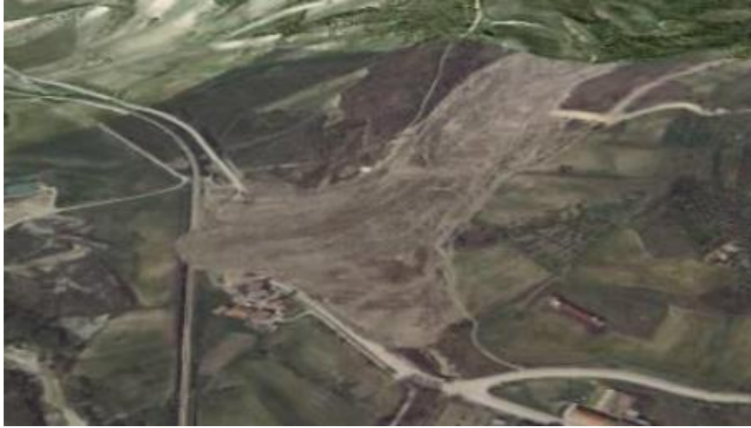
Figure 20 - Landslide toe covering the road SS90 and railway after 2010 movement (source: Guerriero, Revellino, Grelle, et al. , 2013)
