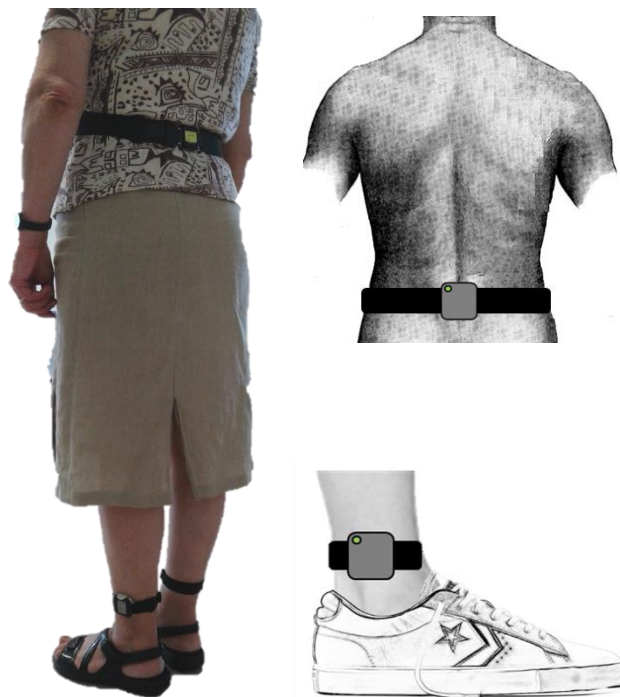
Figure 4-2 Individual with PD wearing the MIMUs on the left; MIMU positionings above the ankles and at L5 level on the right
