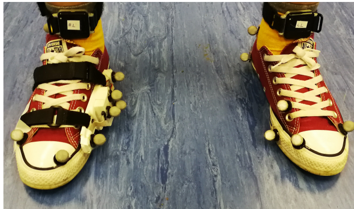
Figure 6.4 – Markers positioning during the initial static calibration acquisition. The marker positioned on the fifth metatarsophalangeal joint was not considered in the data analysis of this study.
