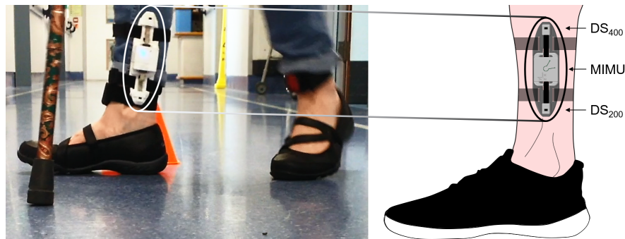
Figure 8.4 – A patient with multiple sclerosis wearing the SWING 2DS system positioned above the right medial malleolus with the DS pointing to the contralateral leg.
