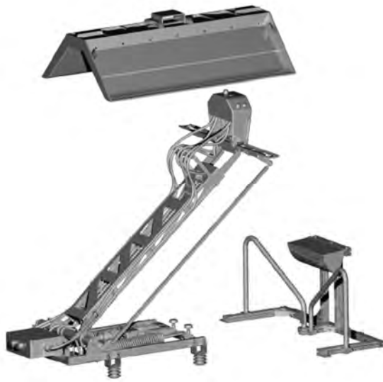
Figure 13 A pantograph used to connect vehicle to overhead electric lines (made by Shunk)
