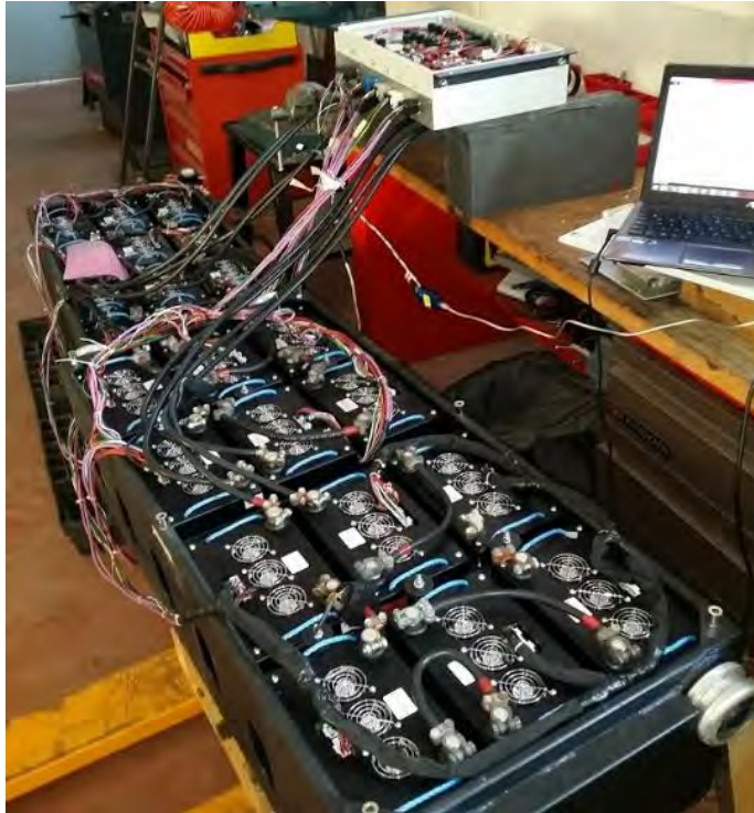
Figure 10 The prototype of ESS used in project “minibus with fast charge policy”
