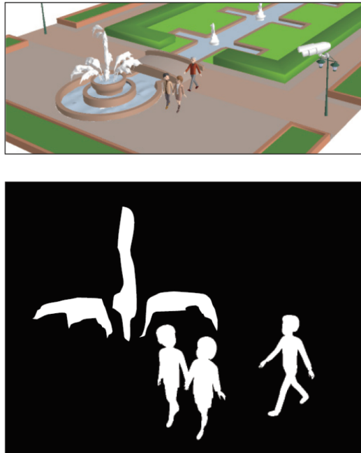
Figure 1.8. Example of false positive in change detection algorithms. The fountain is part of the background, but since it is moving is detected as a change.
