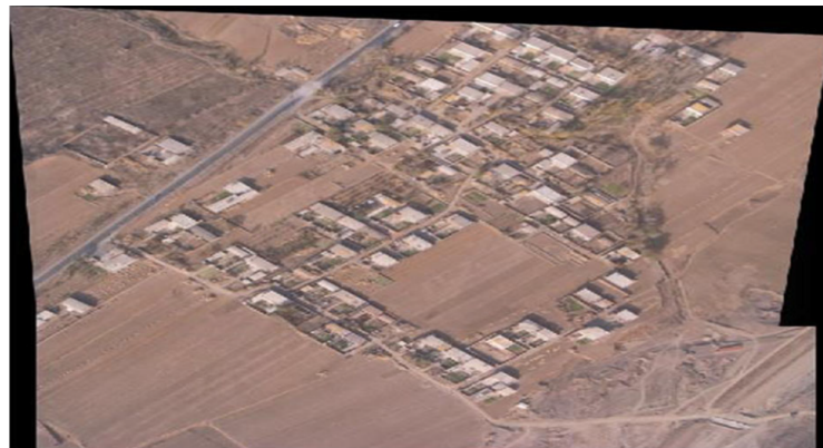
Figure 1.4. Example mosaic obtained with GA-SIFT and O-RANSAC.
