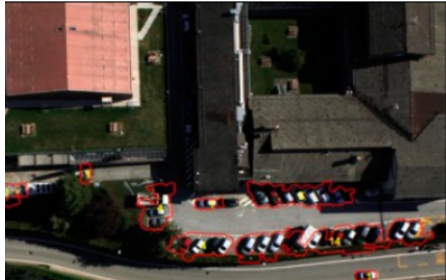
Figure 1.12. Detection of cars in UAV imagery by using CNN and SVM.
