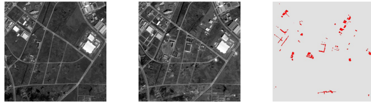
Figure 1.9. Result of the improved binarization proposed in [107].
