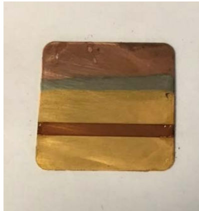
Fig. 3.16. The photo shows a 100 nm layer of nickel so that the gold produced can not be contaminated, in the galvanic process, with a copper substrate.
