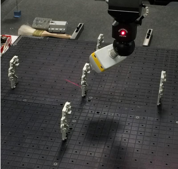
Figure 8. The laser scanner in use during the measurement of a series of components.
