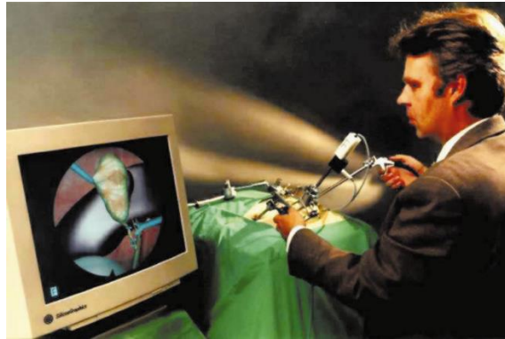
Figure 2.3. The MIS training system for VR-based simulation of the cholecystectomy (Reproduced from [22])
