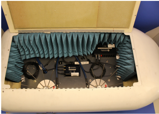
Fig. 6.2: Image of the measurement equipment: The pod, two spider elements (at the bottom), IMU, and RAM to prevent hardware damaging from a strong direct signal.
