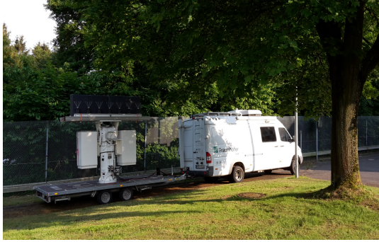
Fig. 4.13: The van with the array on the caravan.
