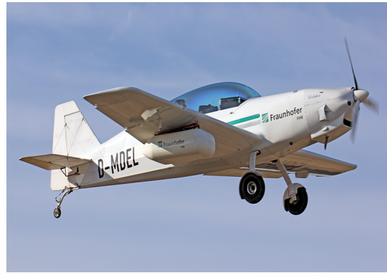
Fig. 6.3: The ULA with the pod mounted below the right wing.
