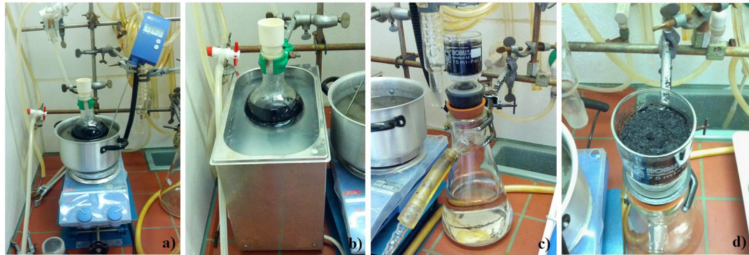
Figure 4.2: Liquid-phase oxidation treatment of the MWNTs consisting of a) the magnetic stirring, b) ultrasonic bath, c) filtering, washing and d) drying.
