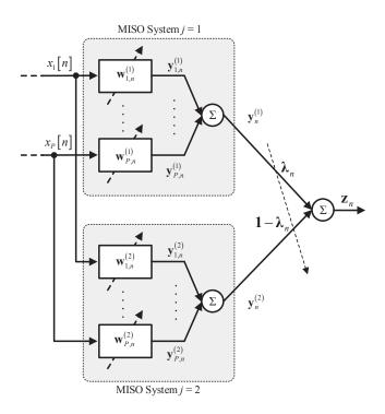
Figure 1. System-by-system combination scheme of two adaptive MISO filters.
