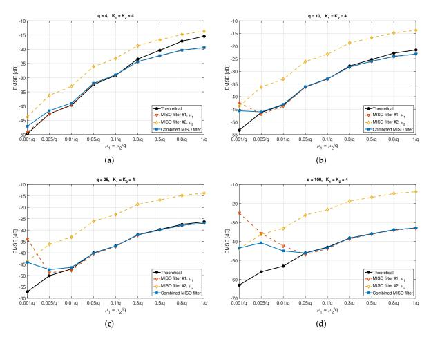
**Figure 2.** Steady-state theoretical and measured excess mean squared error (EMSE) for a combined MISO filter using different step-size values, according to  $\mu_1 = \mu_2/q$ , with (a) q = 4, (b) q = 10, (c) q = 25, and (d) q = 100.
