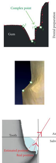
Figure 22 Complex points and critical surfaces during intraoral scanning effects (Raphaël R, Goujat A, Venet L, Viguie G, Viennot S, Robinson P, Farges JC, Fages M, Ducret M. Intraoral Scanner Technologies: A Review to Make a Successful Impression. Journal of Healthcare Engineering 2017; 1-9).
