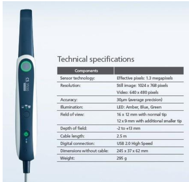
Figure 23 Technical specifications of Intraoral Scanner Carestream 3500®.
