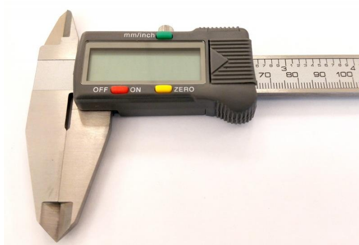
Figure 26 Digital Caliper used in the in vivo measurements for the comparisons with the digital measurements.
