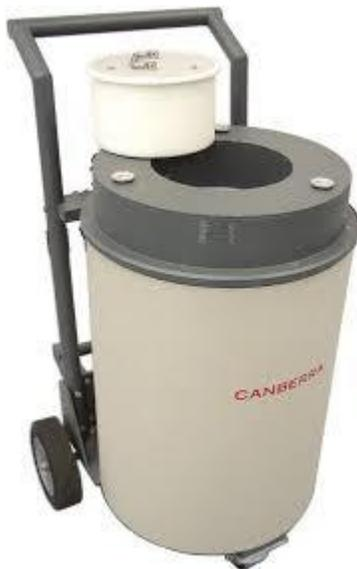
Figura 2-9 – Esempio di active coincidence counter: Canberra JCC-51.
