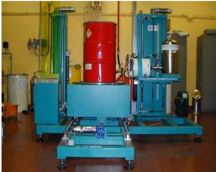
Figura 2-4 – Segmented gamma scanner.
