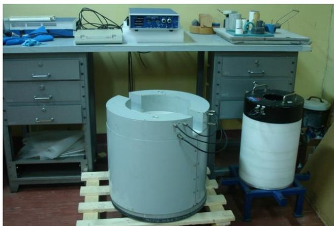
Figura 2-7 – SSNC Small Samples Neutron Counter.
