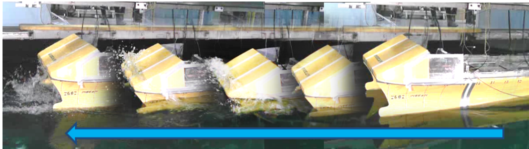
Figure 3.2: Slamming illustrated by combining five consecutive frames to provide an impression of the event in time.
