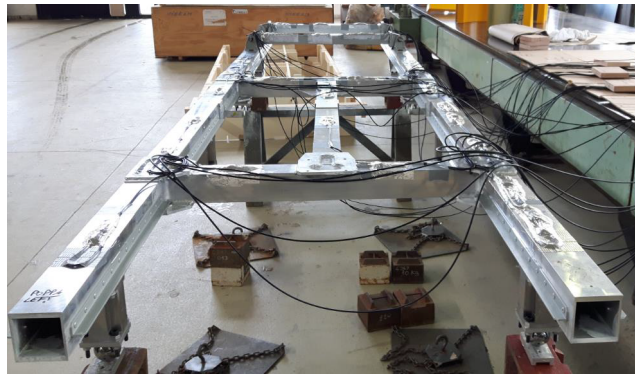
Figure 3.8: Static experimental tests for strain gages calibration assessment.
