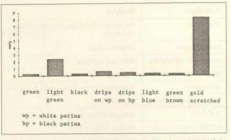
Fig. 5. Average values of the rate of corrosion in various areas of the horse different as to colour
