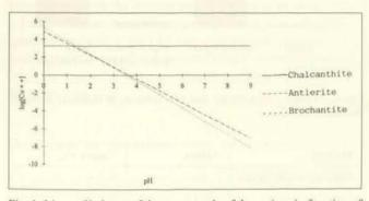
Fig. 1. Lines of balance of the compounds of the patinas in function of the pH and of the concentration of copper ions for a 0.1 ppm concentration of sulphate ions (the compound is stable above its line of balance)
