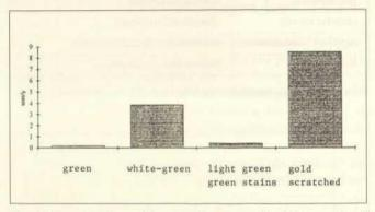
Fig. 6. Average values of the rate of corrosion in different areas of the rider
