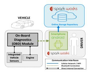
Fig. 3: System Architecture
