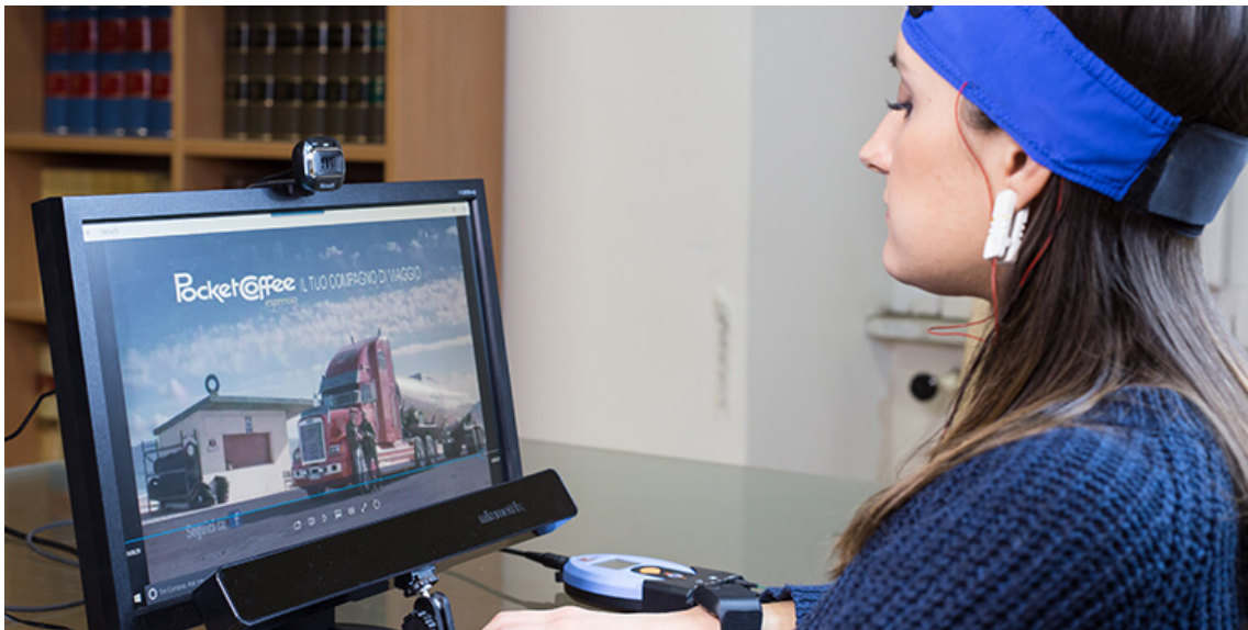
Figure 13 – The picture shows the experimental set-up of a neuromarketing study. The subject - whose cerebral activity is gathered by a lightweight and portable device (the EEG acquisition device) - is seated in front of a computer screen on which a neutral documentary is running. Usually is inserted a series of commercial breaks within, each consisting of several TV advertisements, which will be the stimuli in test.
