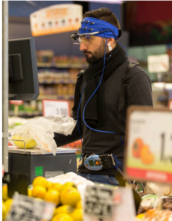
Figure 12 – The picture shows the experimental set-up during the visit of a food retail (Shopping Experience). The experimental subject wears a cap with the electrodes, and the cerebral activity is gathered by a lightweight and portable device (the EEG acquisition device). The subject wears also an eye-tracker device to detect eye-movement during the exploration of a goods.
