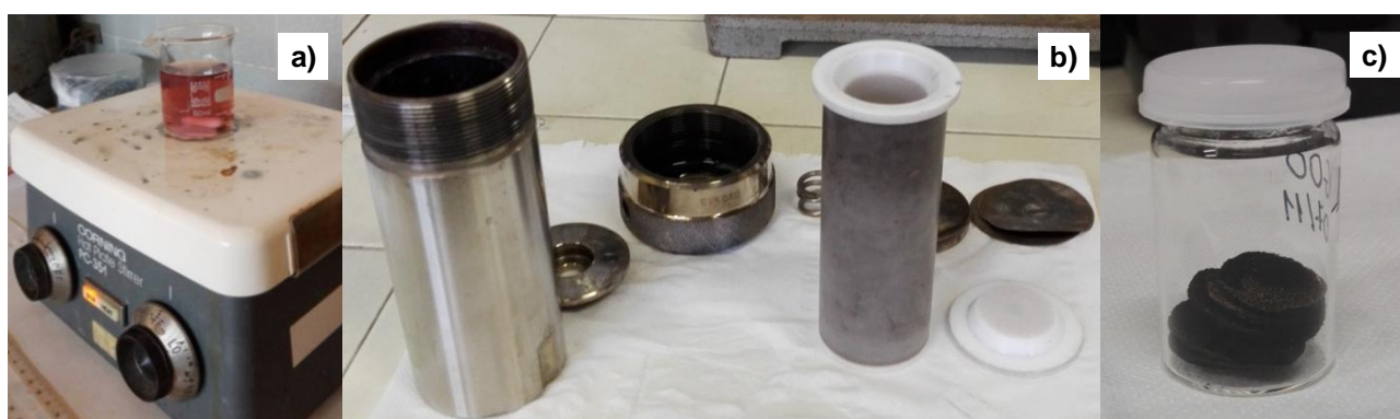
Figure 20. (a) The pink aqueous solution of the nickel cobaltite precursors and urea under magnetic stirring; (b) the Teflon lined stainless autoclave used for the hydrothermal synthesis; (c) the obtained composite discs of \text{NiCo}_2\text{O}_4 on Ni foam.
