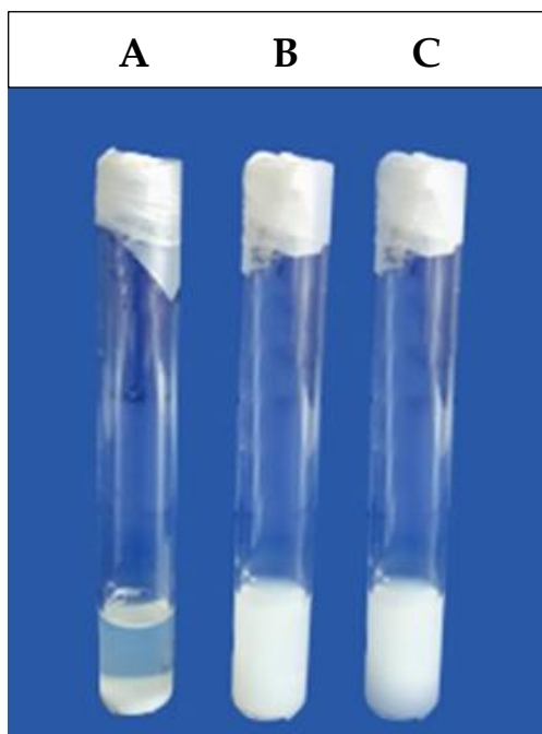
Figure 7.3. Different colloidal stability of CL (A), GiLUV 750 (B) and GiLUV 4000 (C), after 14 days from the liposomes preparation. All samples were stored at 4 °C.
