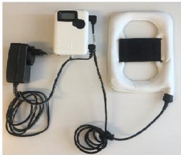
Figure 4.1. I-ONE coil exposure set-up with the generator, the power supply and the solenoid.
