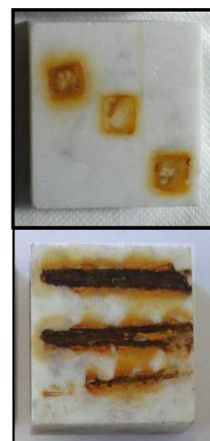
Fig. 1; Carrara marble stained by iron cubes (above) and nails (below)
