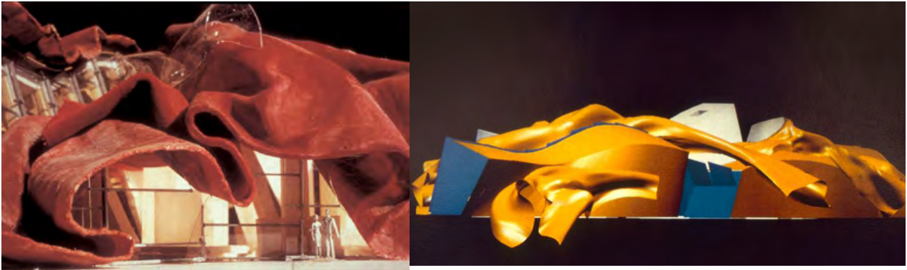
Figure 4. The Lewis Residence by Frank Gehry, Lyndhurst, Ohio (1989-1995). The pin bars, plexiglass and wax/velvet cloth model and the CATIA spline drawing.
