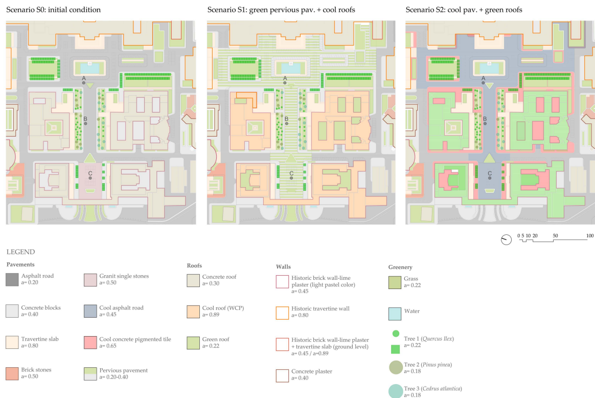
Figure 6. Initial condition scenario S0 (a), first renovation scenario S1 (b), second renovation scenario S2 (c). Point A, B, and C represent the selected location for the comparisons among the scenarios.
