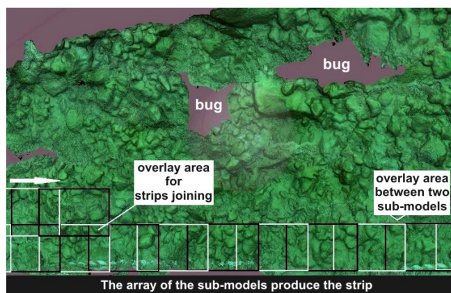
Figure 11. Overlap of sub-model Mesh and strips generation (modified from [9]).
