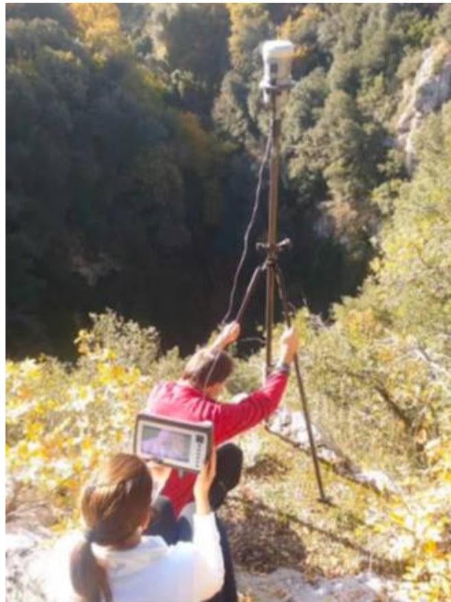
Figure 1. The imaging rover combined with GPS/GNSS receiver (on top) during the survey of “Pozzo del Merro”.
