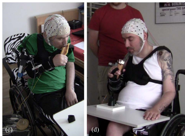
Fig. 6. Subfigure (a) Overview of the hBCI control of the upper extremity neuroprosthesis. Subfigure (b) Control scheme of the neuroprosthesis: A short imagination of a movement of the right hand switches between shoulder and elbow control. A long imagination switches to or from a pause state. Subfigure (c) End user with high cervical spinal cord injury and no voluntary finger, hand, and elbow function uses the hBCI-controlled hybrid neuroprosthesis to eat a pretzel stick. Subfigure (d) Same end user eating an ice cream cone.
