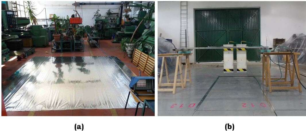
FIG. 1 – (a) Experimental setup for a 400 MHz ground-coupled antenna in a laboratory of the Faculty of Technical Sciences, in the University of Novi Sad, in Serbia. (b) Experimental setup for 1 GHz and 1.8 GHz air-coupled antennas in a laboratory of the National Laboratory for Civil Engineering of Lisbon, in Portugal.
