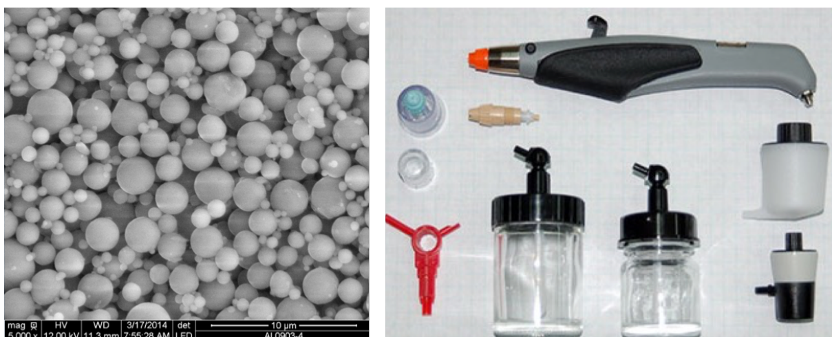
Figure 4.18: Aluminum microparticles purchased from Hermillion (France) on the left; aerograph on the right
