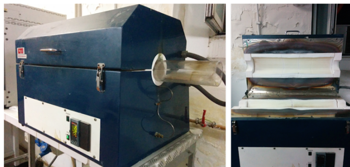
Figure 4.5: Tubular furnace Lenton Thermal Design Ltd, with quartz reactor.
