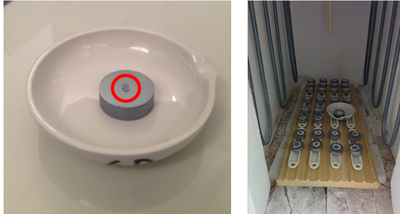
Figure 4.8: Hot corrosion test procedure: slurry application on a sample (left, red circle) and samples prepared for the heat treatment (right)
