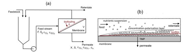
Figure 1: Schematic illustration of flows and quantities relevant to biofouling build-up in the adopted macroscopic context (a) and in the control volume (b).
