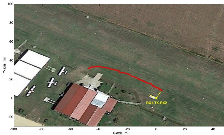
Figure 36. Test against a small maneuvering aircraft: (a) picture of the performed test; (b) Wi-based PBR localization results.
