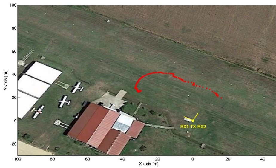
Figure 35. Test against a maneuvering aircrafts: (a) picture of the performed test; (b) PBR results compared to the available ground-truth.
