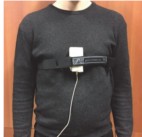
FIGURE 1: The piezoelectric belt and the UWB radar antenna.
