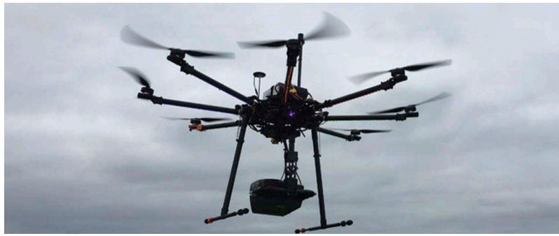
Figure 1. Remotely Piloted Aerial System carrying the LiDAR.
