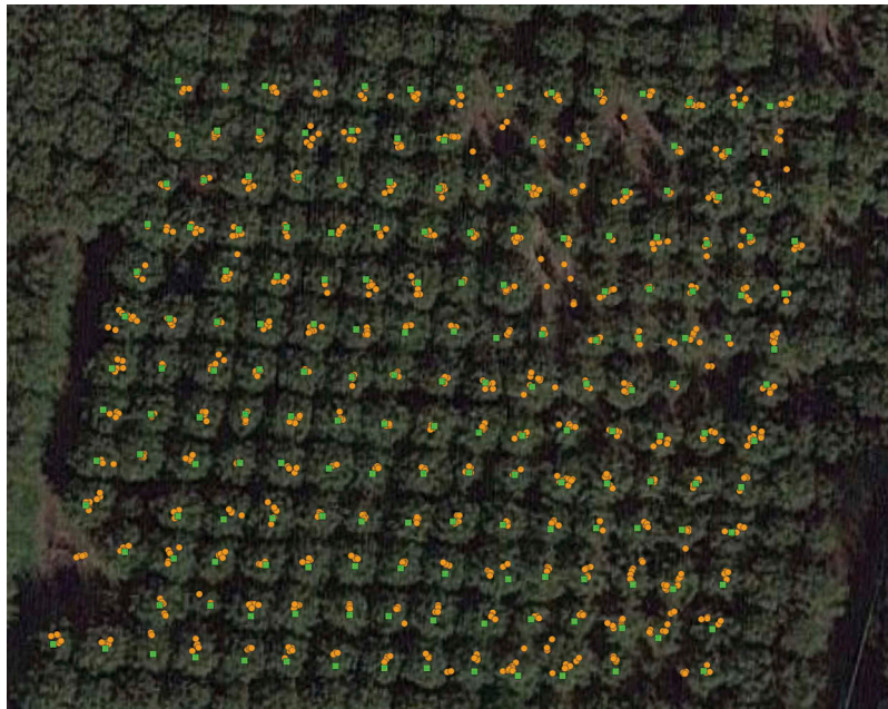
Figure 16. Orthophotograph of the hazel grove considered in this work. Ground truth is represented by green squares denoting tree centers, while orange points represent RANSAC results.
