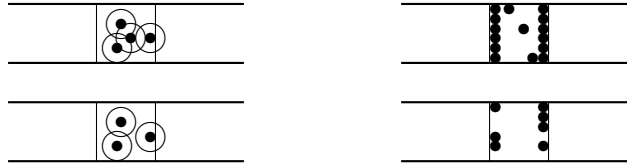
FIG. 1. Sketch of pedestrians moving through a cell of the obscure tunnel driven by a two-threshold biased dynamics. Left: The smaller filled circles represent the individuals located inside a cell; the bigger circles encompassing the smaller black ones represent the interaction range of each individual. For an efficient communication network to be settled, a certain overlap among the bigger circles is needed, which is hence guaranteed by requiring that the number of individuals in the cell exceed the activation threshold A . Right: As soon as the front row of the cell is full, the number of individuals occupying that front row, corresponding to the saturation threshold S , fixes an upper bound to the escape rate from the cell.
