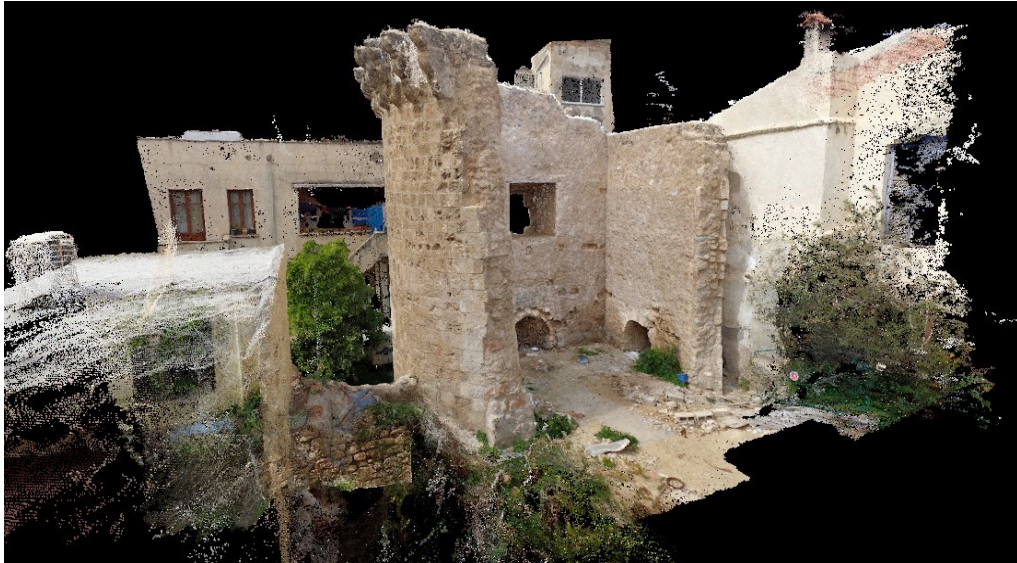
Fig. 9- A rendered view of the 3D model (Griffo, 2018)
