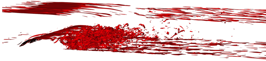
Figure 3. Instantaneous vorticity surfaces at constant magnitude.
