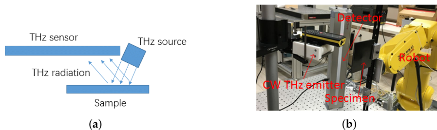
Figure 7. CW THz configuration in reflection mode: (a) schematic set-up; (b) experimental set-up.
