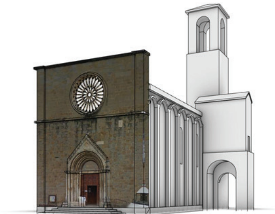
Figure 19. 3D model of the Church of St. Agostino in Amatrice. The elevation is textured by projecting the equi-rectangular image from the Google panorama.
