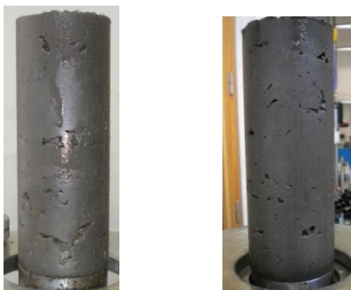
(a) Tapping (b) Static Compaction
