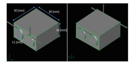
**Figure 2.** Swirling combustor converter, Z/D = 3, 2 connected chambers.
