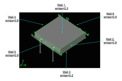
**Figure 5.** Swirling combustor converter, Z/D = 11-5 chambers, emissivity values.
