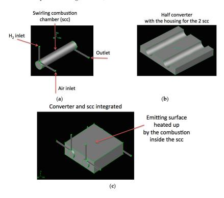
**Figure 1.** Swirling chamber (**a**); half thermal conductive brick (**b**); and integration into the energy converter (**c**).
