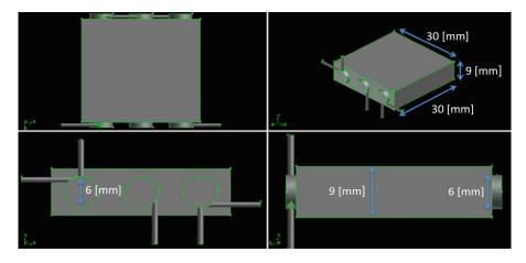
**Figure 3.** Swirling combustor converter, Z/D = 5, 3 connected chambers.
