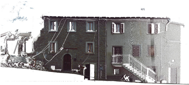
Fig. 5. Photoplan of the 3D model taken from the point cloud (image by Leonardo Paris).
