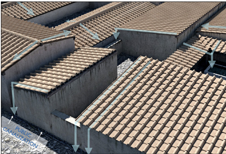
Fig. 4 – Reconstruction of the roofing and the water disposal system of the Houses 2 and 3 of the Regio IV, 1 .
