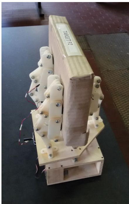
Figure 15: Example of an experiment with a prismatic target (P2). Right plot shows the contact forces.
