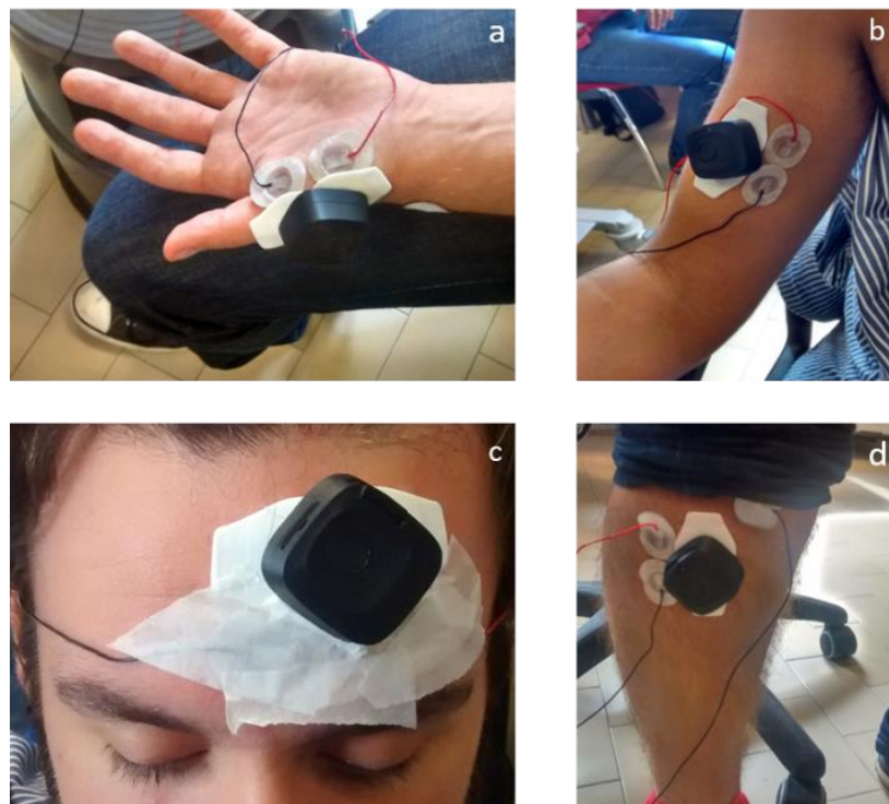
Figure 8. Placement of Digitimer D360 and Bio2Bit surface electrodes on the: (a) abductor pollicis brevis muscle; (b) biceps brachii muscle; (c) frontalis muscle; and (d) tibialis anterior.
