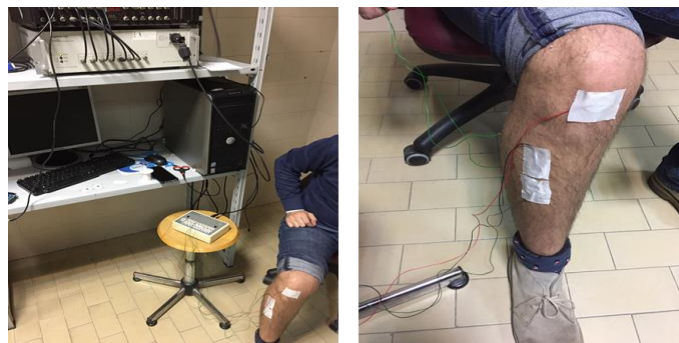
Figure 7. Typical set-up of a sEMG with a conventional wired equipment that is used in biomedical research laboratories.
