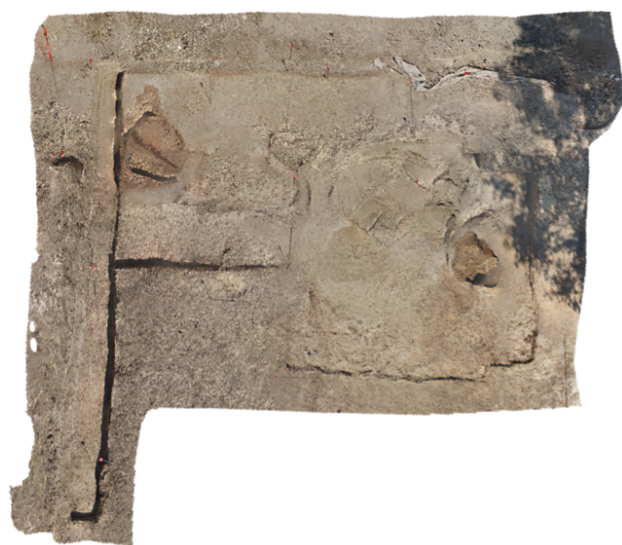
Figure 4: elevation model by CRP and TLS surveying (excavation campaign 2013)
